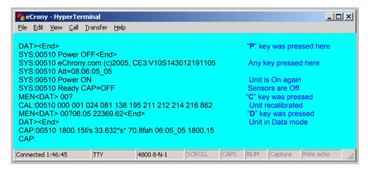
b) **Normal mode** – press "D" to go to Data mode and from there press "C" to calibrate. In this mode CE-3 will decide for you if the environment is acceptable and enable sensors accordingly. Please note: CE-3 has a limited intelligence and may not always be right.
